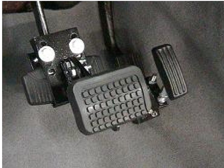
Figure 3.6. Brake and Gas Pedal Extensions
