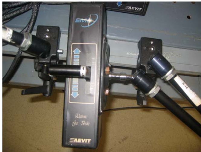
Figure 4.10. Electronic Gas and Brake Device
