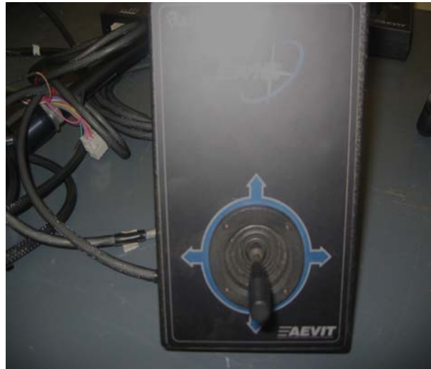
Figure 4.7. Digital Joystick of the AEVIT System
