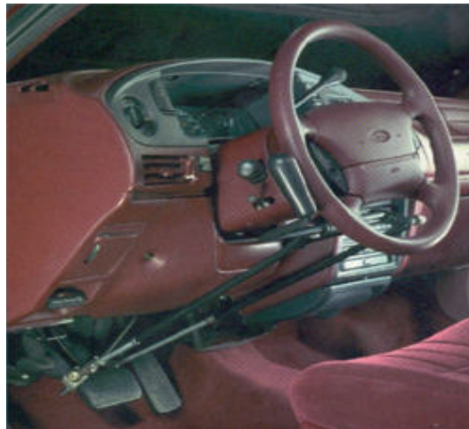
Figure 3.5. Sure Grip Mechanical Hand Control
