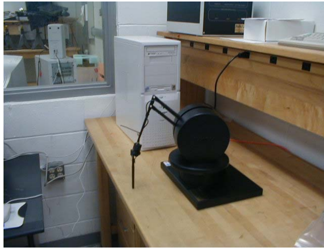
Figure 4.1. PHANTOM Haptic Device by Sensable Technologies Inc
