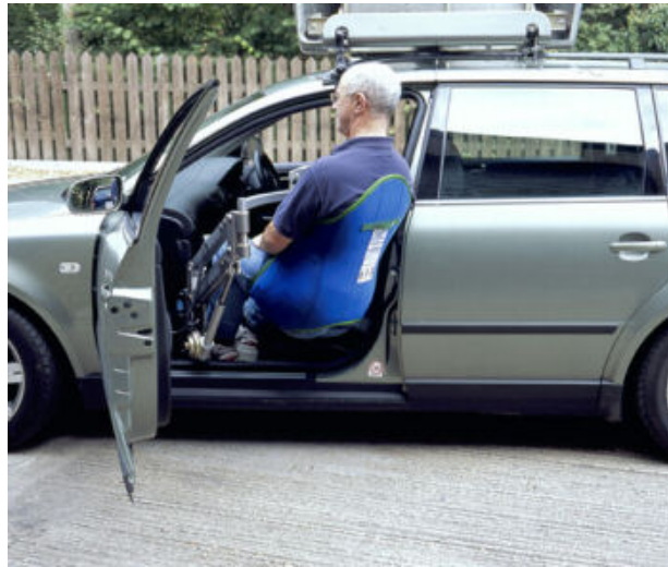
Figure 3.10. Milford Aluminum Electric Person Lift
